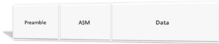
Figure 2.8: iNET Packet Structure
