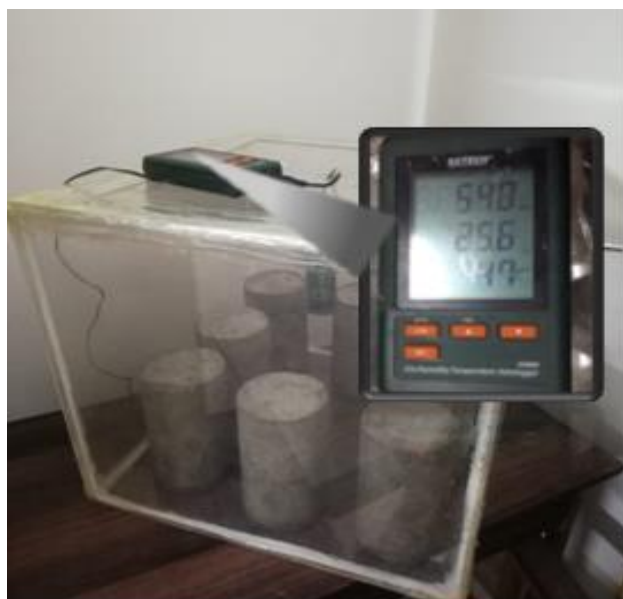
Figure 32: Real time CO 2 monitoring in the climate control chamber
