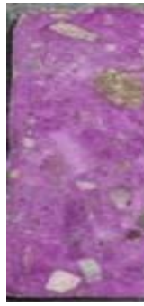
Figure 36: Phenolphthalein test for BZ
