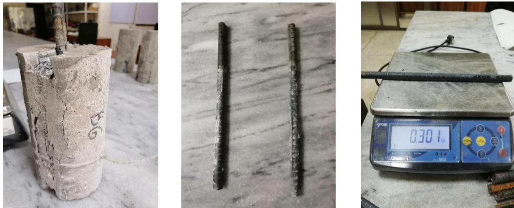
Figure 29: Pictorial description of weight loss measurement test
