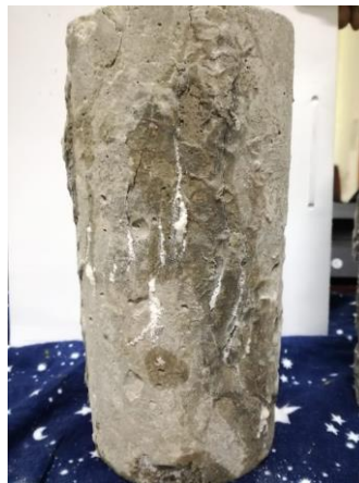
Figure 38: Autonomous healing of BZ repaired sample in 2 nd cracking cycle
