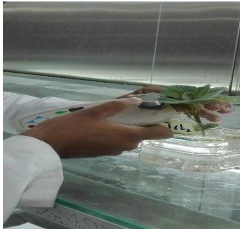
Figure 3.5: Chlorophyll estimation using CCM-200 plus Chlorophyll meter
