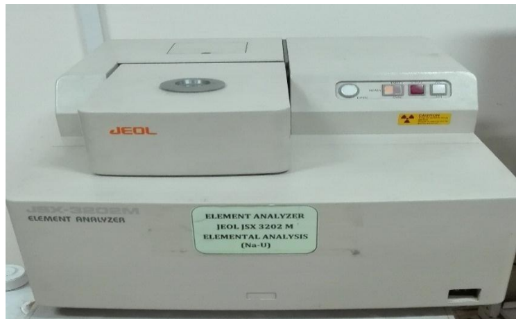
Figure 3.8: X-ray Fluorescence Spectrometer (JEOL JSX-3202-M, Japan)
