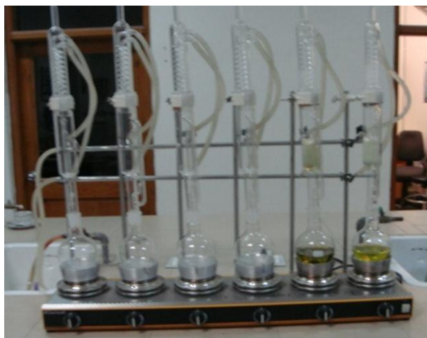
Figure 3.7: Soxhlet apparatus for oil extraction (Gerhardt - 1712-08-0069) at IESE-NUST
