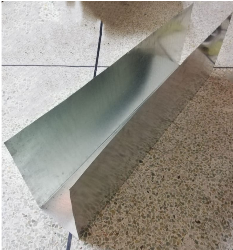
Figure 7. Zinc Coated U-Shaped Steel Plate
