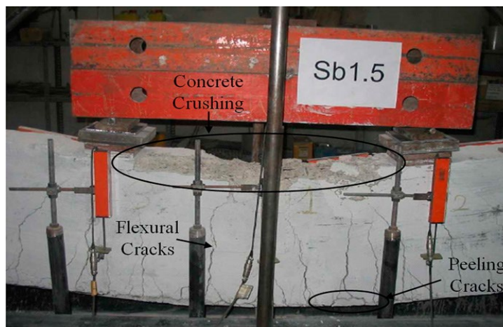
Figure 3. Peeling Failure
