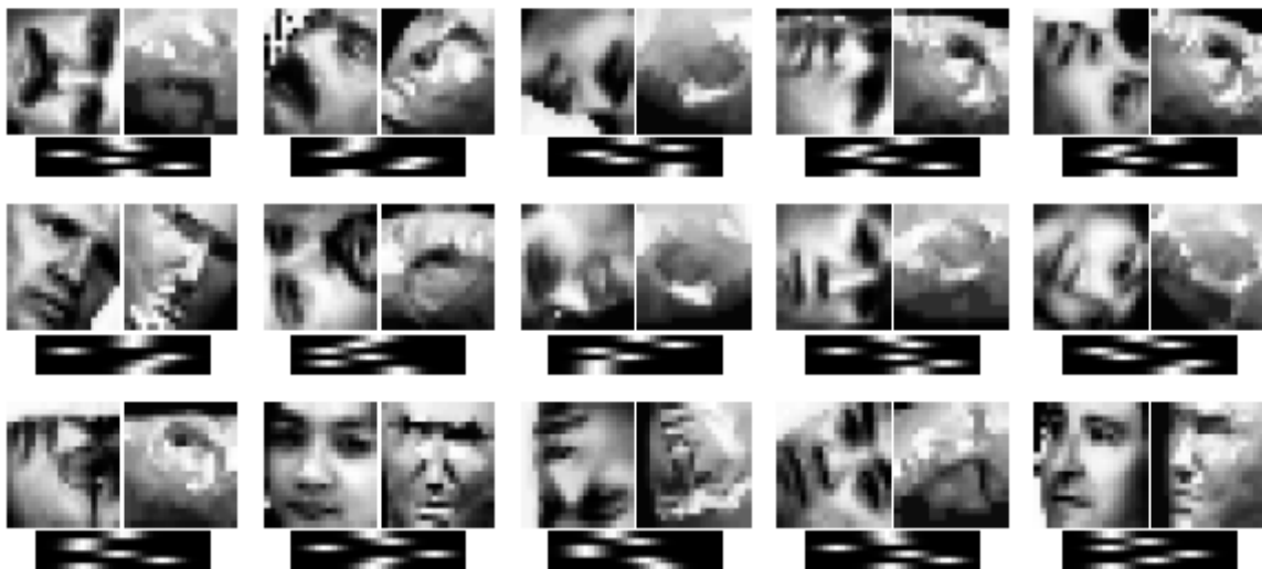
Figure 7.4: Example input images (left) and output orientations for the pose estimation neural network. The pose is represent by six vectors of output units (bottom), collectively representing 6
