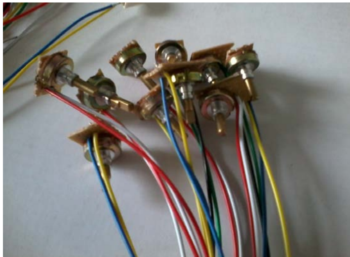
Figure 3-5: Potentiometers Used in the Exoskeleton
