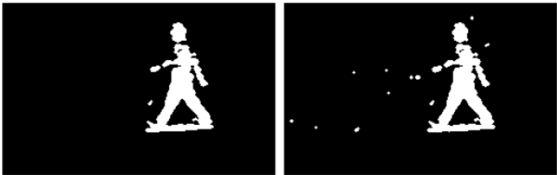
Figure 4.4 Blob Size Thresholding
