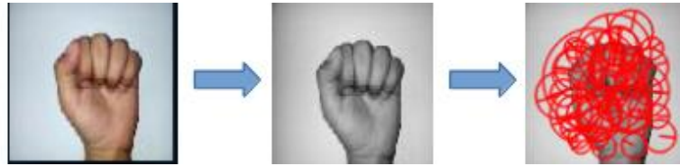
Figure 3.2: SURF Key-point extracted from grayscale image
