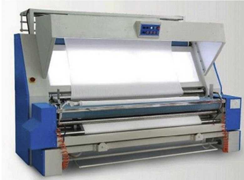
Figure 1: Quality Inspection Fabric machine [3]
