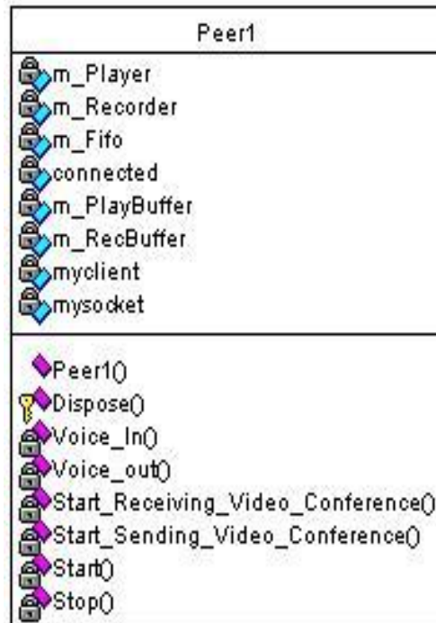
Figure 19: Class diagram of Audio/Video Module
