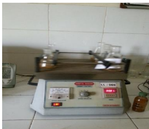
Figure 3: Orbital shaker used during the experimental work for shaking the adsorbent and leachate solution for different contact times.
