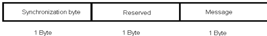
Figure 5.4 Control Message Structure From Base Station To Visual Sensor Node
