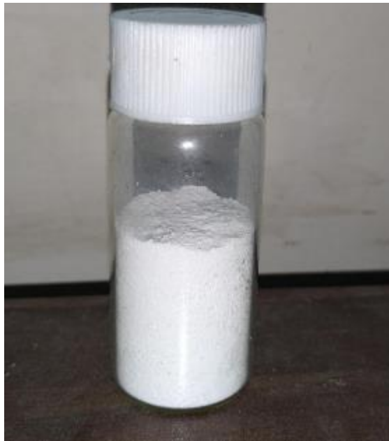
Figure 3.22 Glass Powder after high energy ball milling
