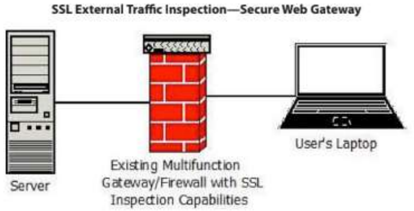
Figure 6: External Traffic Inspection
