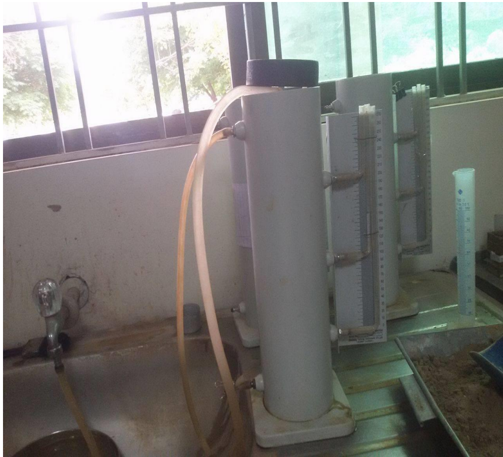
Fig 13: Constant Head Test Performed in Geotech Lab, NICE
