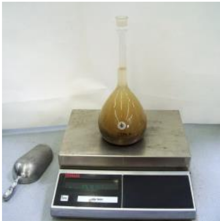
Fig 12: Specific Gravity Apparatus
