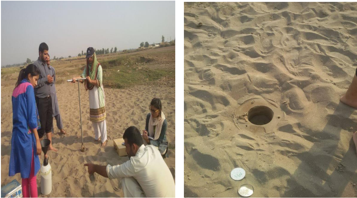
Fig 9: Sand Replacement Test at Site
