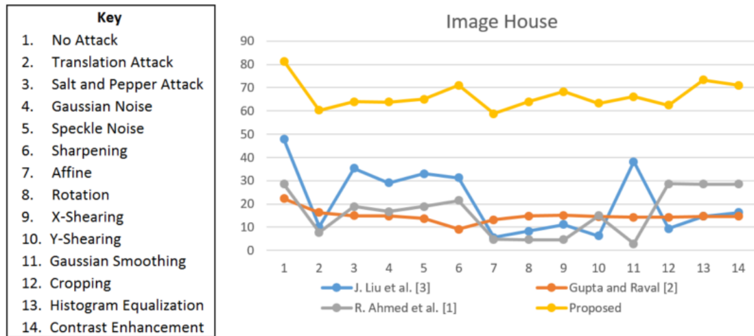
Figure 4.8 PSNR value comparison of the suggested technique with Ramsha et al. [1], Gupata and Raval [2] and J. Liu et al. [3] against all attacks using image “House”
