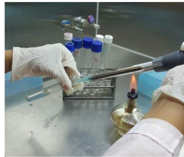
4. Serial dilution in saline solution
