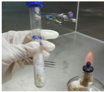
1. Fabric sample transferred into test tube containing MRSA culture
