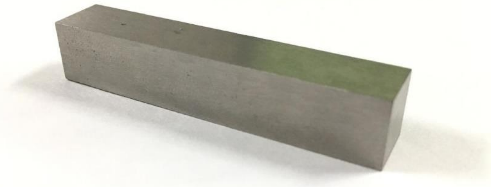
Figure 21. Machined unnotched Charpy impact testing sample of HIP sintered W-HEA
