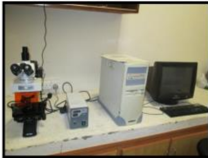
Figure 3.7: Fluorescent microscope for visual analysis (Model No. Optika, B-350, Italy).
