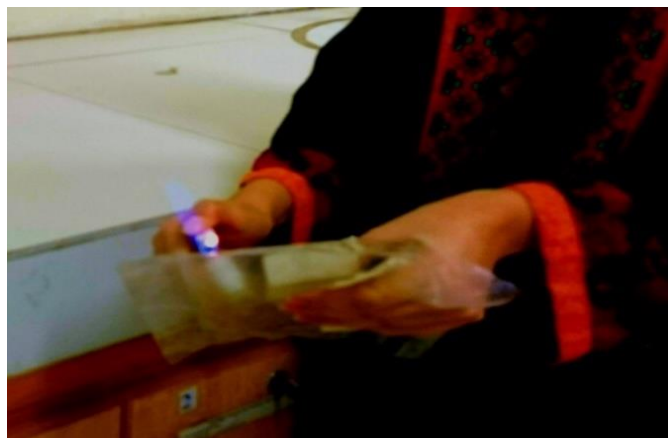
Figure 19: Methane gas analysis through flame test
