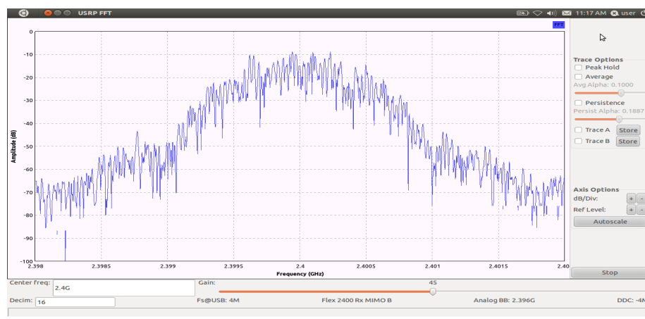
Figure 3.1-10: FFT plot MIMO GMSK link
