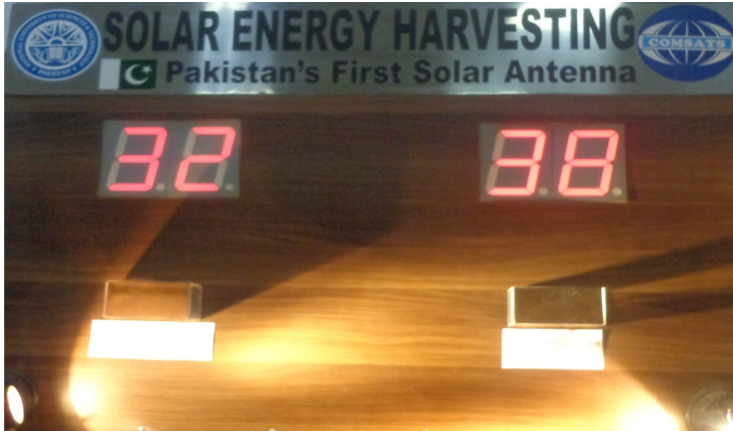
Figure 6.2 Testing of solar antenna array: Temperature after Heat Source is applied
