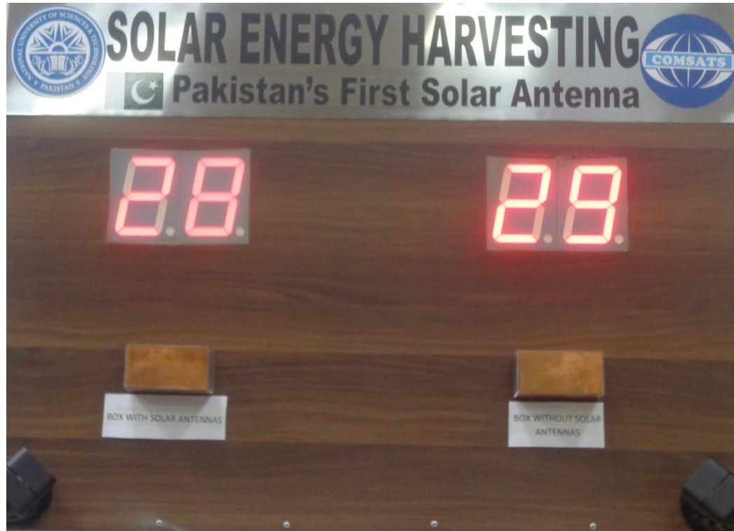
Figure 6.1 Testing of solar antenna array: Temperature before Heat Source is applied
