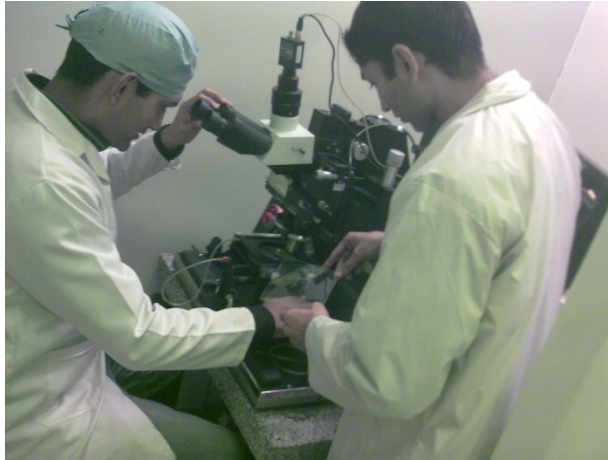
Figure 1.2 Calibration of Photolithography machine in clean room
