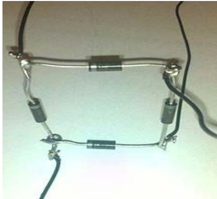
Figure 3-5 Simple Diode bridge configuration
