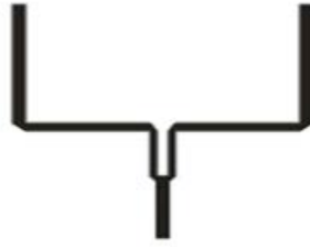
Fig 6.6 one to two power divider
