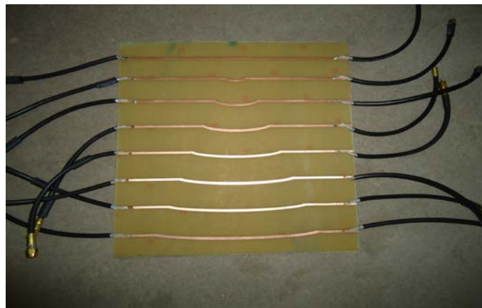
Fig 7.3 Manufactured Beam former
