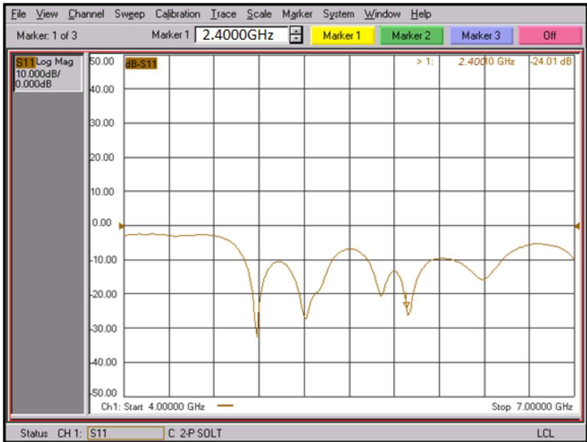
Fig. 7.4 Return Loss of Beam former
