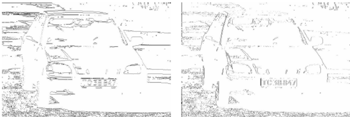
Figure 2-3: Horizontal and vertical edges
