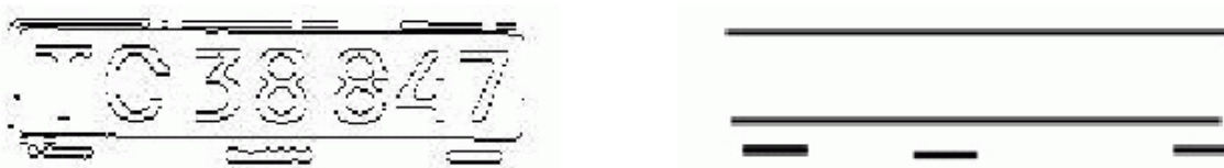
Figure 2-5: Example license plate and reconstructed line segments
