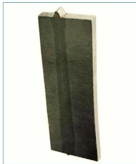
100 mm thickness titanium butt weld
