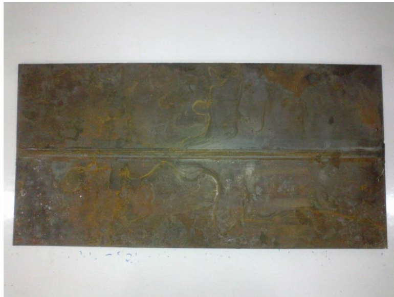
Fig.5.4 TIG welded Test coupon after welding on machine
