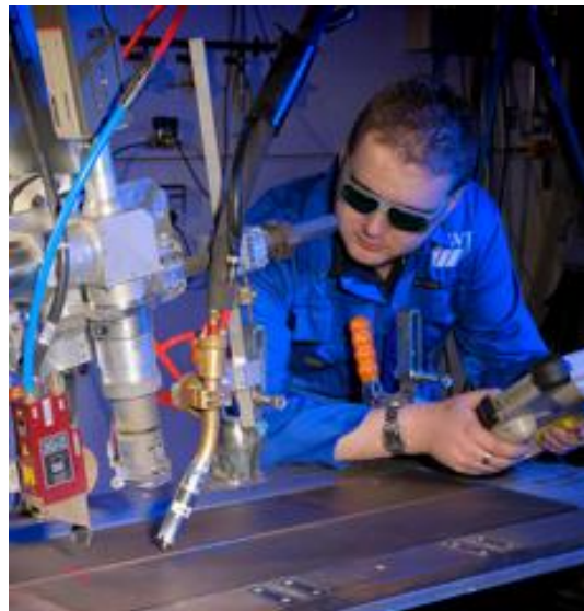
Fig. 1.1 Hybrid Laser Arc Welding [20]
