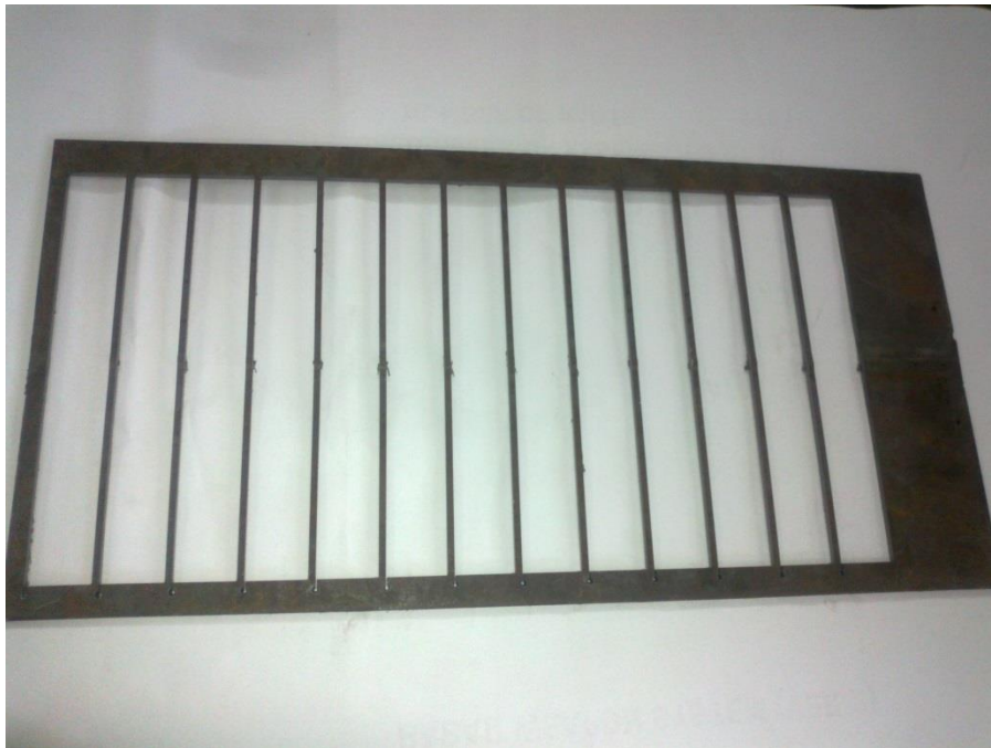
Fig. 5.5 Remainder of test coupon after cutting of sample blanks
