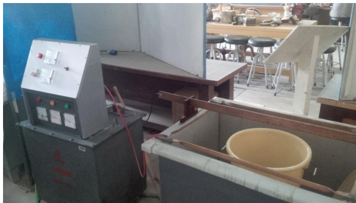
Figure 6 Rectifier and electroplating tank
