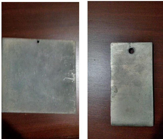
Figure 5 These pictures are of low current and high time values. Only burning occurred.
