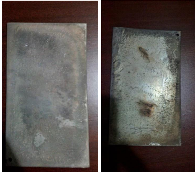
Figure 4 These pictures are of high current and too much time applied. Blistering and burning occurred.
