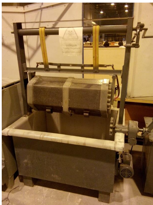
Figure 3: Electroplating Machine in NUST MRC
