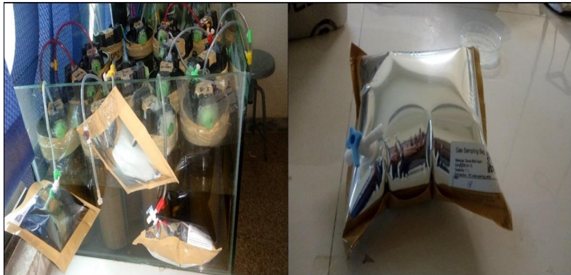
Figure 3.6: Illustration of biogas collection for compositional analysis
