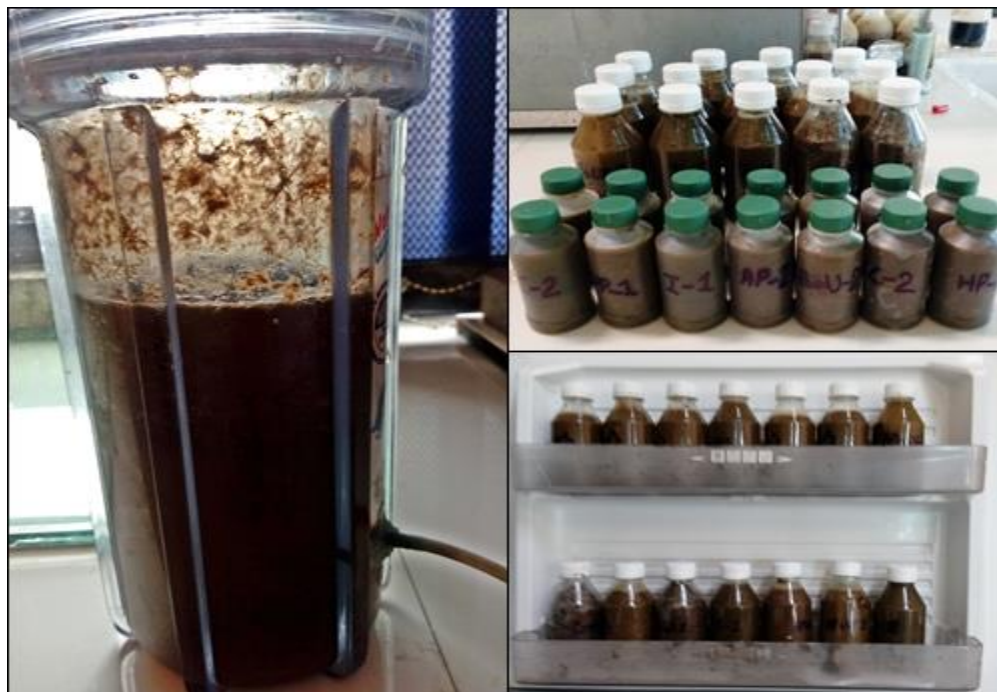
Figure 3.8: Digested slurry collection and storage for analysis
