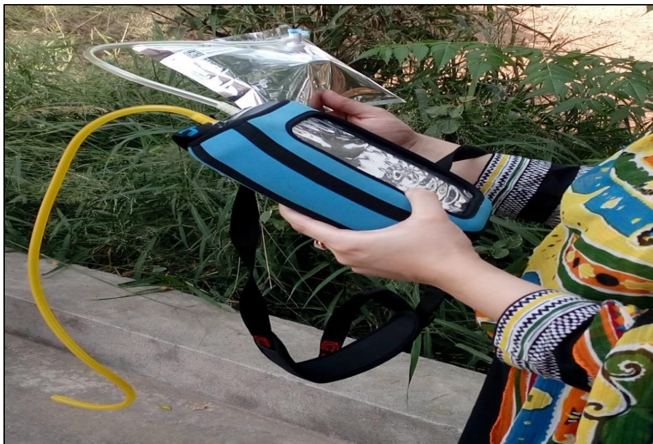
Figure 3.7: Biogas compositional analysis by using biogas analyzer
