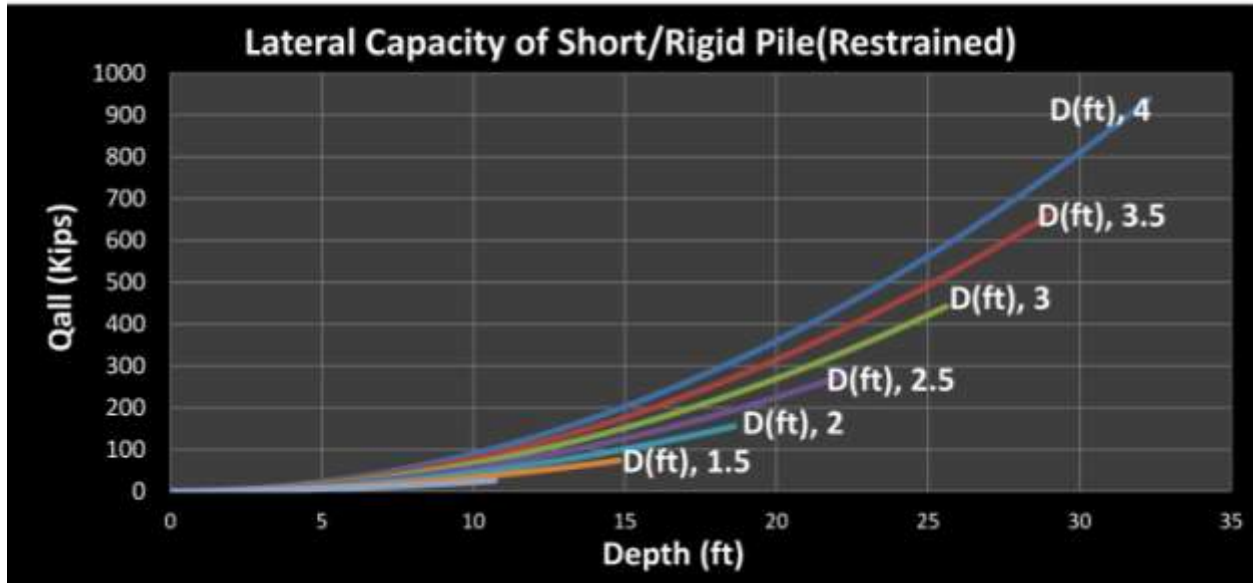
Figure 35: Lateral Capacity of Short/Rigid Pile (Restrained)
