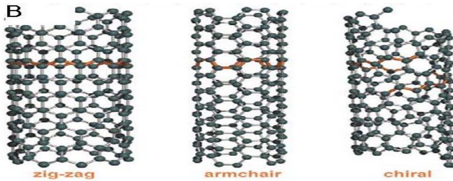
Fig. 2.1-B: showing structure of different nanotubes (a) armchair, (b) Zigzag, and (c) chiral nanotubes (Saito et al. 2002).
