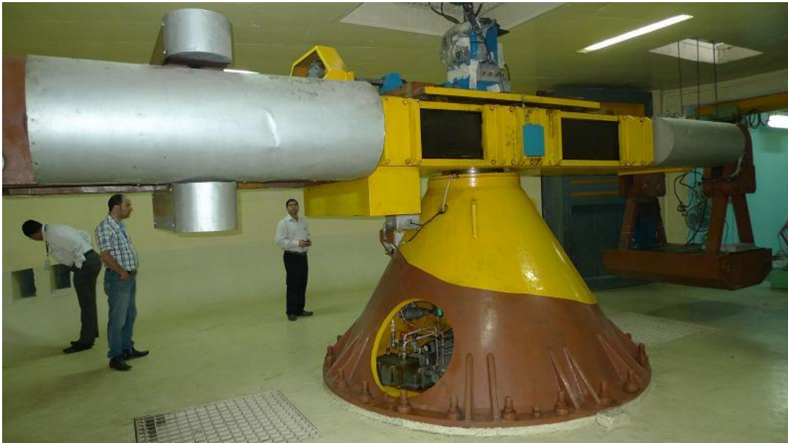
Fig 20: The National Geotechnical Centrifuge facility at IIT Bombay
