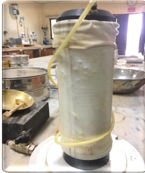
Fig 35: Sample Preparation for the Tri-Axial Test
