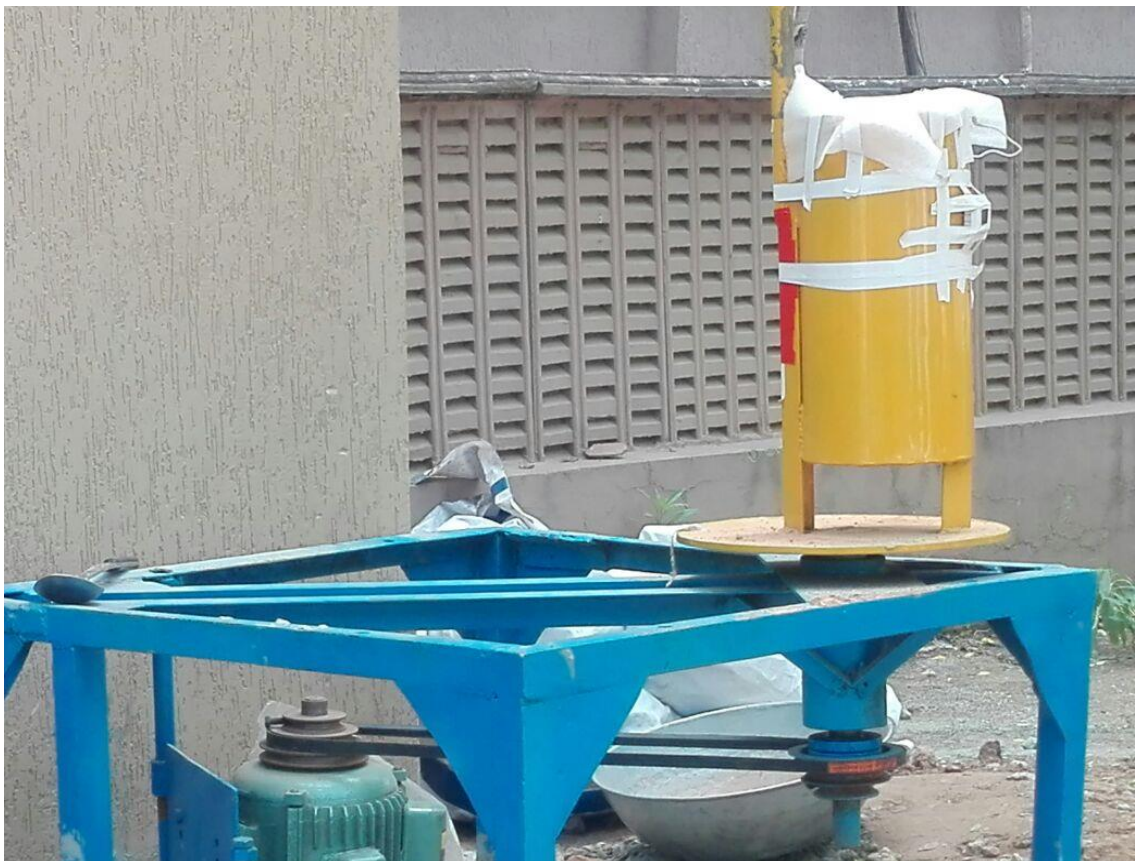
Fig 21: Self-Designed Centrifuge Machine
