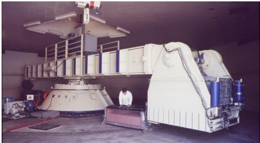
Fig 18: The NEES Geotechnical Centrifuge at UC Davis
