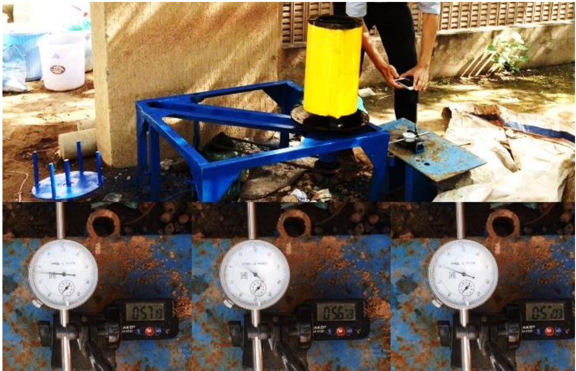
Fig 24: Actual arrangement for recording vibrations
