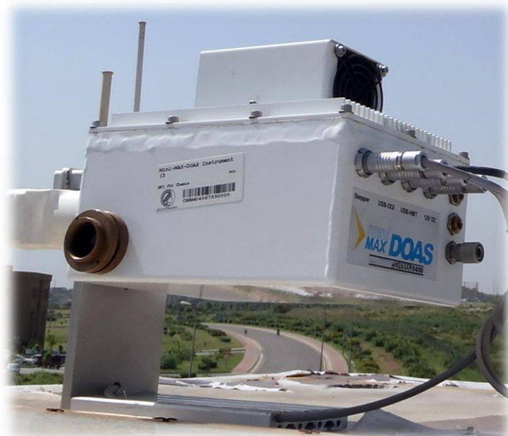
Figure 1.1 MAX-DOAS used in this study
