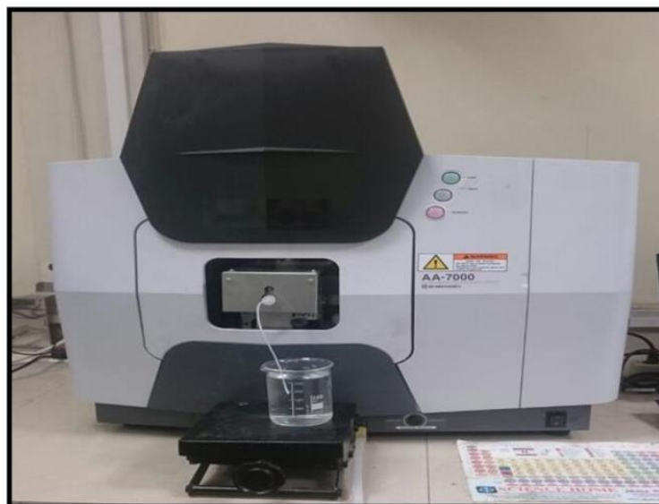
Figure 3.5: Atomic absorption spectrophotometer (AA-7000, Shimadzu).
