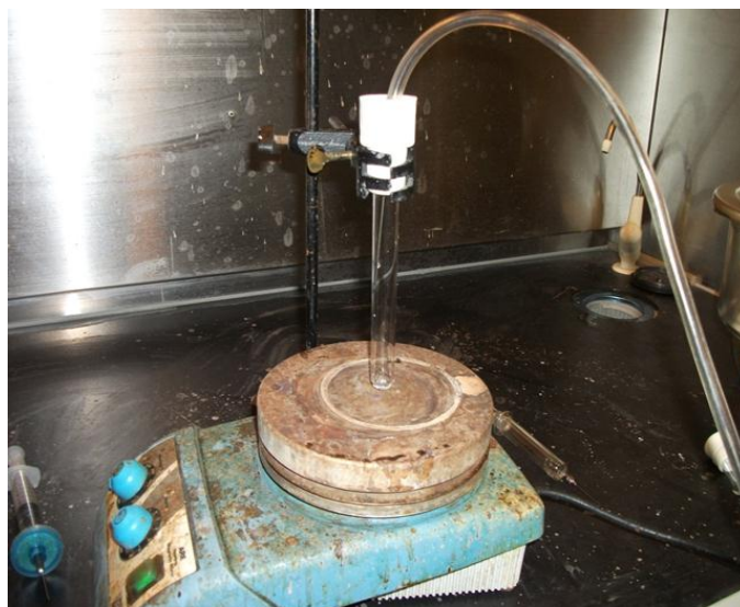
Figure 3.8 Addition of CO 2 through syringe into Grignard's Reagent
