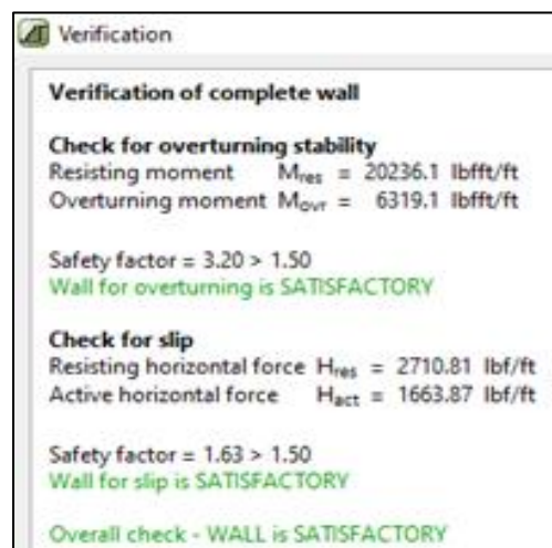
Figure 5.8: GEO-5 FOS for Gabion Walls
