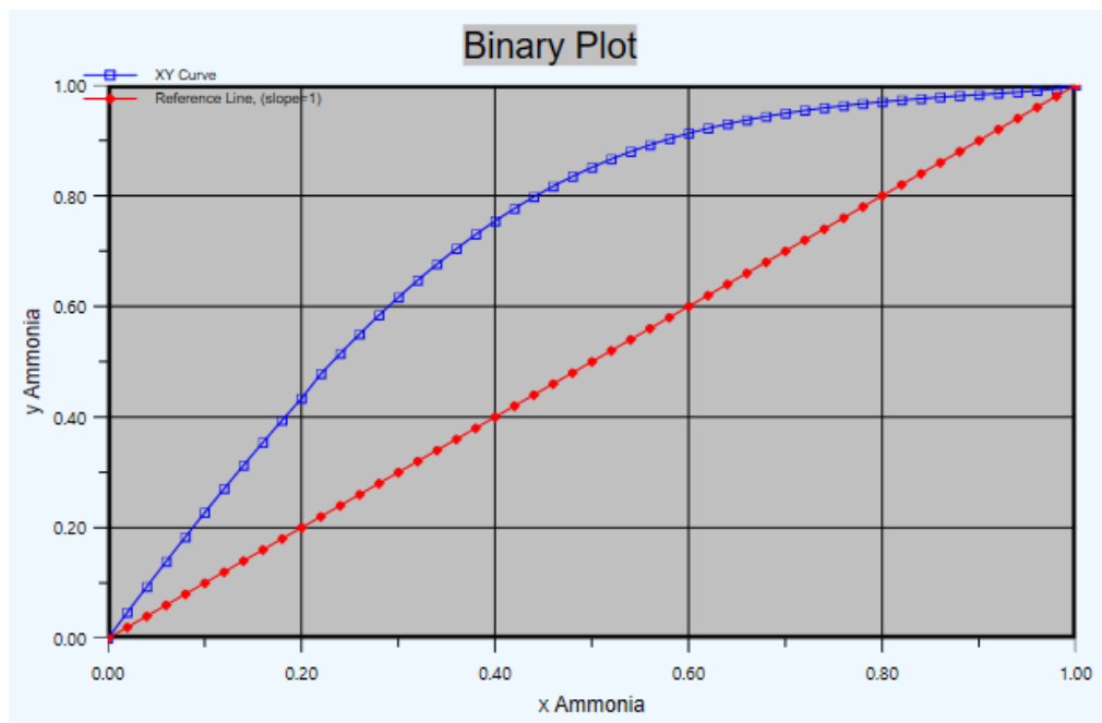
Figure 3 \text{NH}_3\text{-H}_2\text{O} VLE plot (@120bar) from HYSYS (AspenTech Eq Unit)
