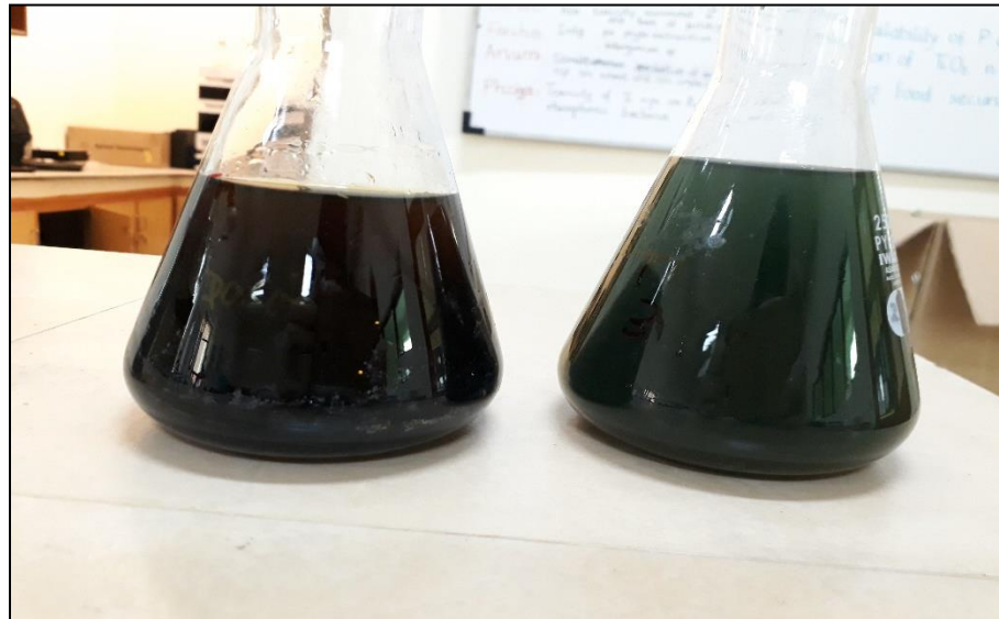
Fig. 3.7. Color changed from violet blue to green in TOC analysis
