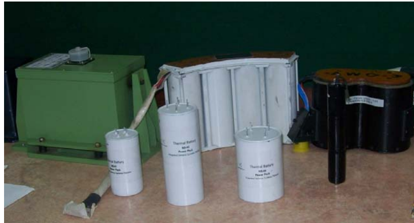
Figure 1.1: Some typical high power lithium thermal batteries in which hermetic glass to metal sealing is employed. The four output terminals made of Kovar bonded with glass seals can be seen. (Courtesy: National batteries Pvt. Ltd. Pakistan)
