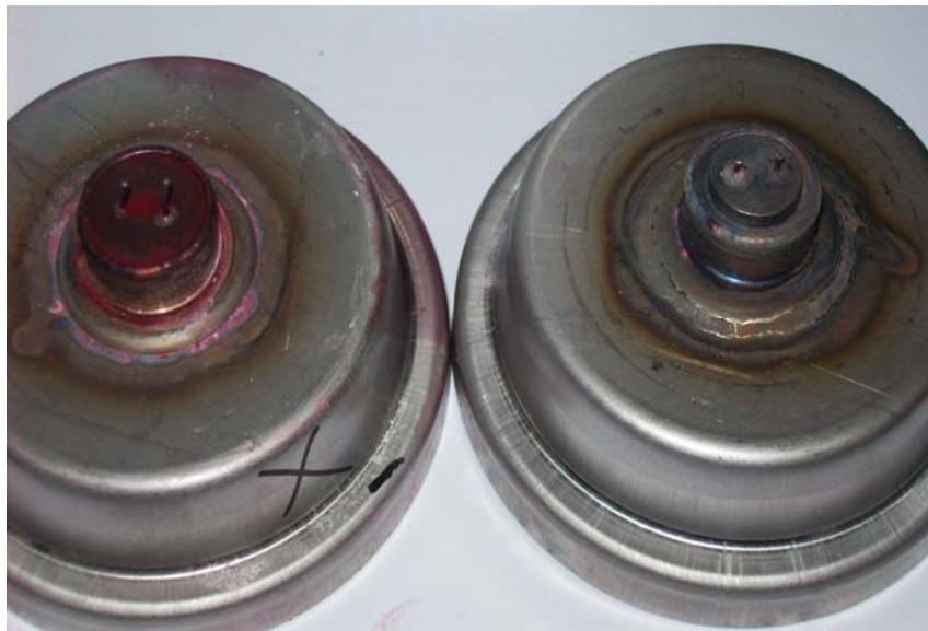
Figure 3.12: The defected vs. un-defected glass-metal seal using the die-penetrate leak test method
