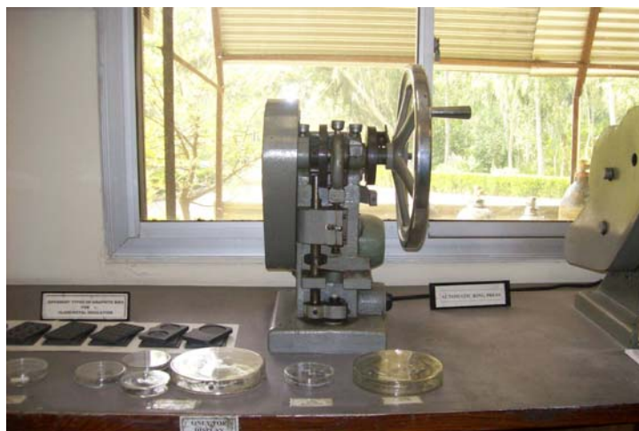
Figure 3.3: The bead forming press that is used to form the green compact of the bead before pre-sintering
