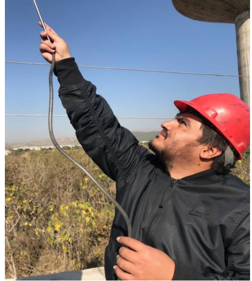
Figure 3.7. Flue gas analysis through flue gas analyser Testo S-350
