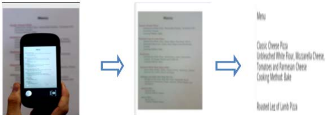
Figure 1 : Text Recognition using Android based mobile phone. (a): Capture image using mobile’s camera. (b): Textual image captured. (c): Recognized text from the captured image.
