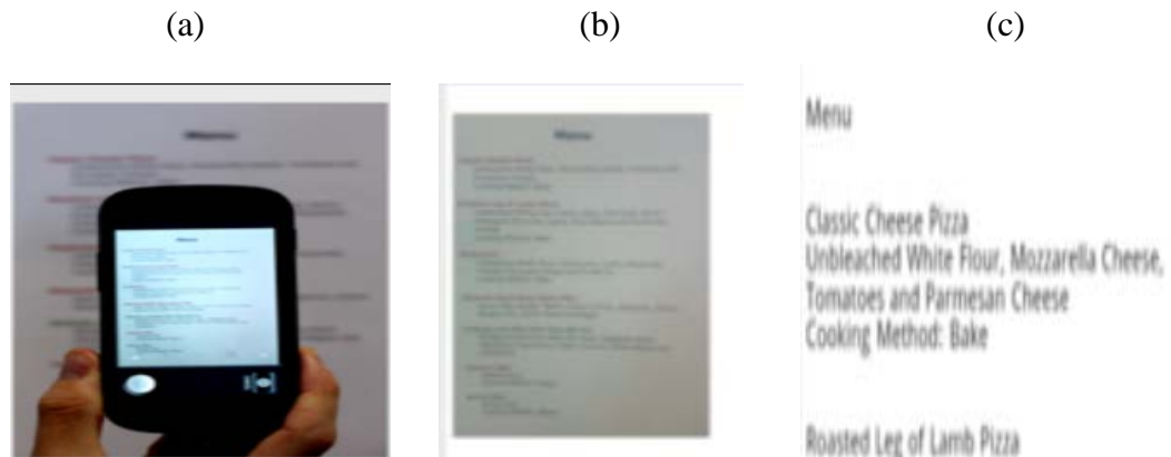
Figure 4 : Text Recognition using Android based mobile phone. (a): Capture image using mobile's camera. (b): Textual image captured. (c): Recognized text from the captured image.
