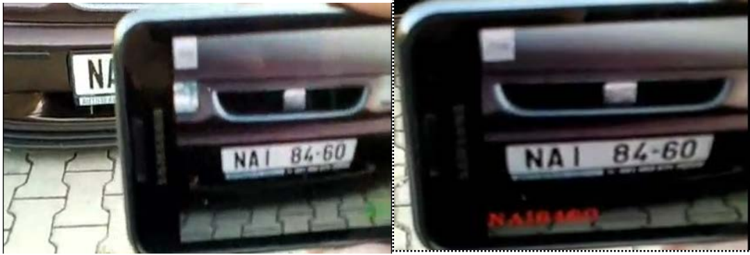
Figure 7: Android based Number Plate recognizer. (a): Number plate image captured (b): Number plate recognized and converted to numeric at the bottom in red color.
