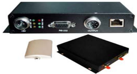
Figure 2.9 Different RFID Reader's interfacing mediums with PC
