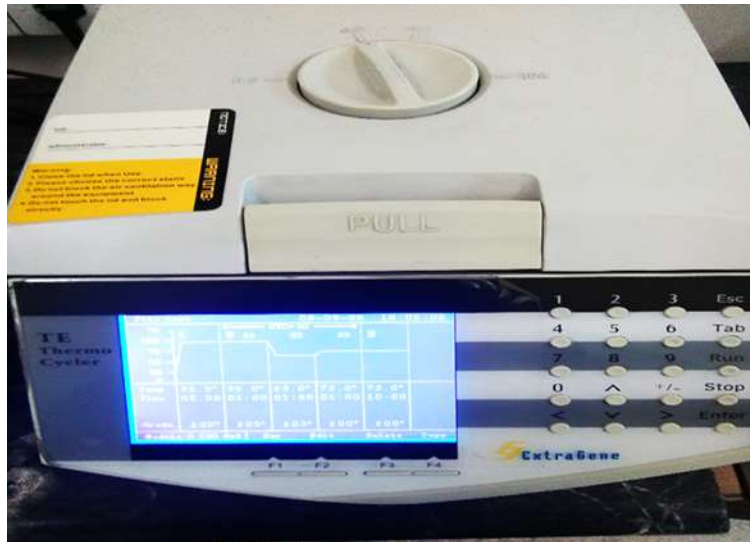
Fig 3.2: Thermal Cycler (Company: Extra Gene 9600)
