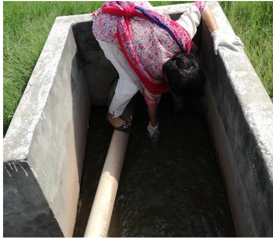
Figure 3.3 Wastewater collection from MBR plant wastewater inlet
