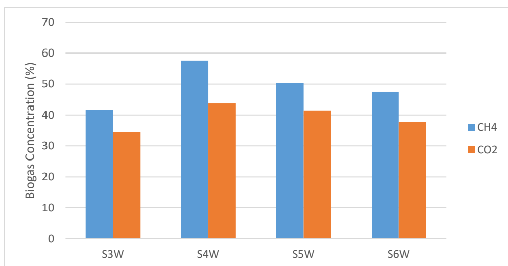
Figure 4.13 Concentration of methane and carbon dioxide in the biogas samples on 15th day
