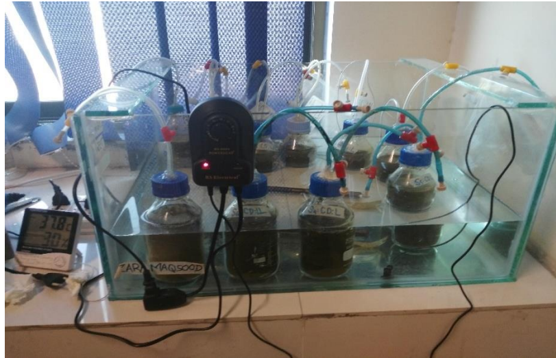
Figure 3.6 Digester bottles dipped in water bath and the temperature is maintained by aquarium heater
