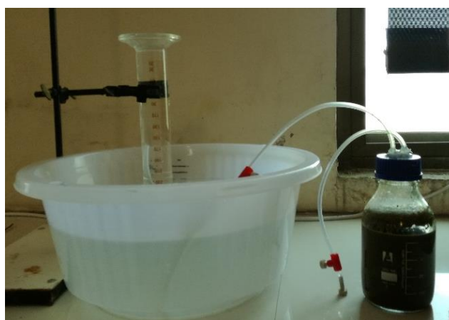
Figure 3.7 Water displacement assembly for measurement of gas
