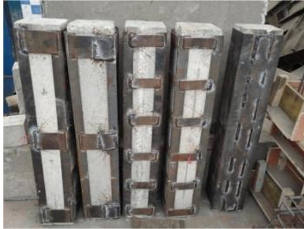
Figure 7. Details of steel jackets for confinement of columns
