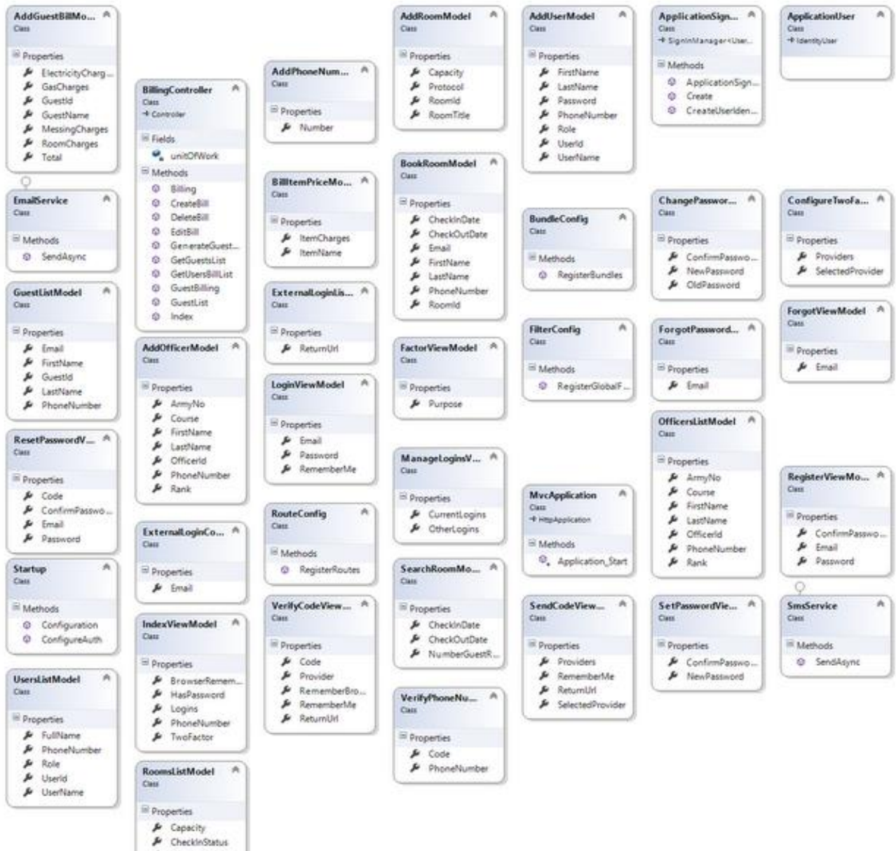
Figure 5 Class Diagram Core Project
