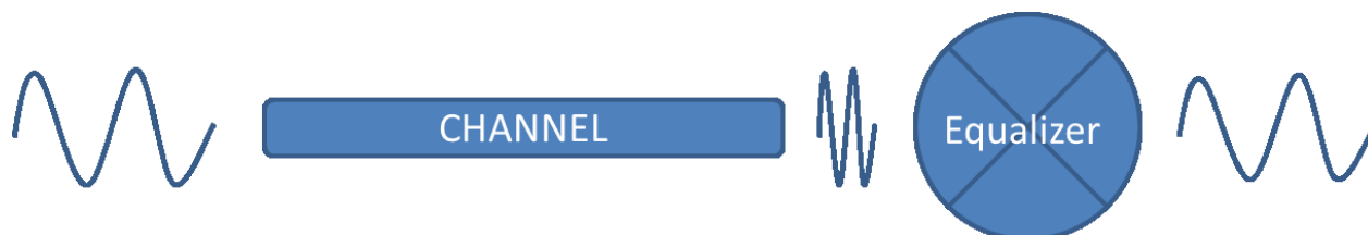
FIGURE 1-1 OVERVIEW OF CHANNEL EQUALIZATION
