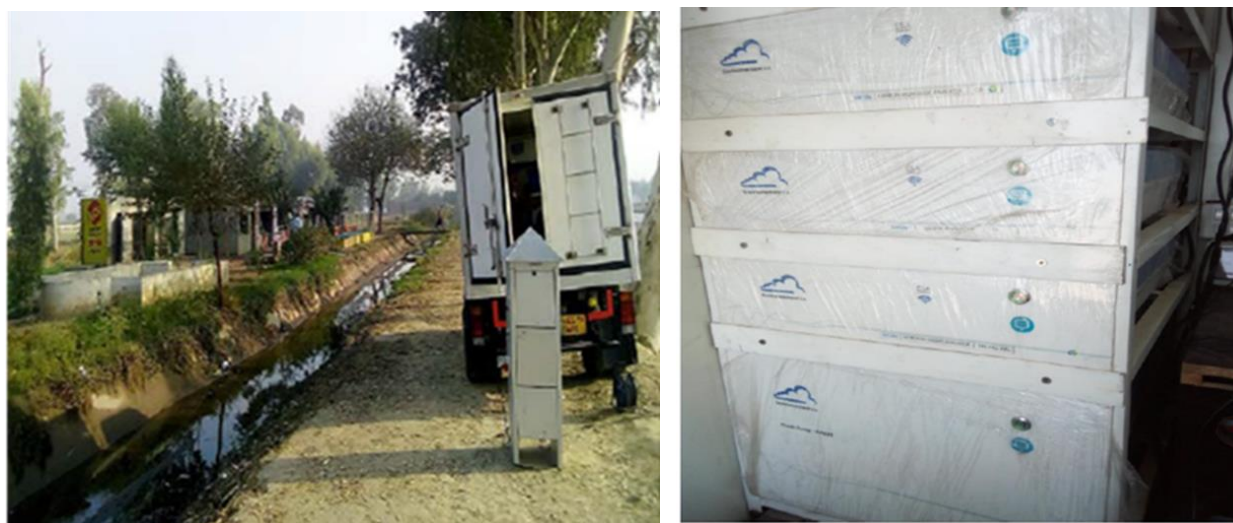
Ambient Air Quality Monitoring Instruments for SPM, PM10, PM2.5, NO, NO2, SO2, CO, O3.
