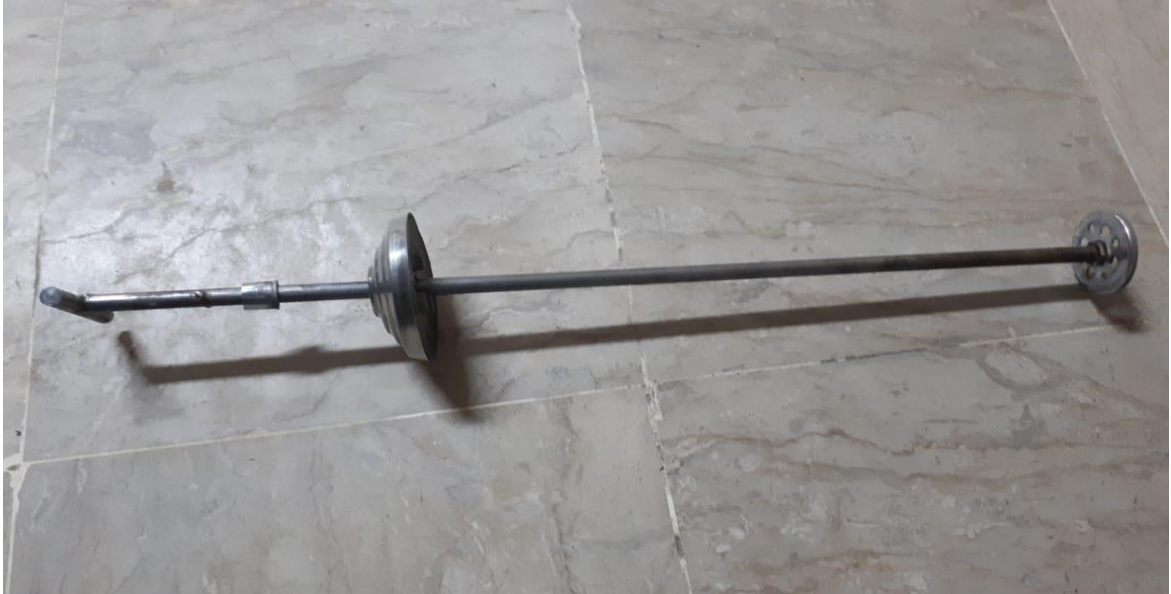
Figure 3.8: Picture courtesy by Malik et al. , 2019 (PCRWR) Controlled length plunger compatible with the standard cylinder for stirring the soil suspension
