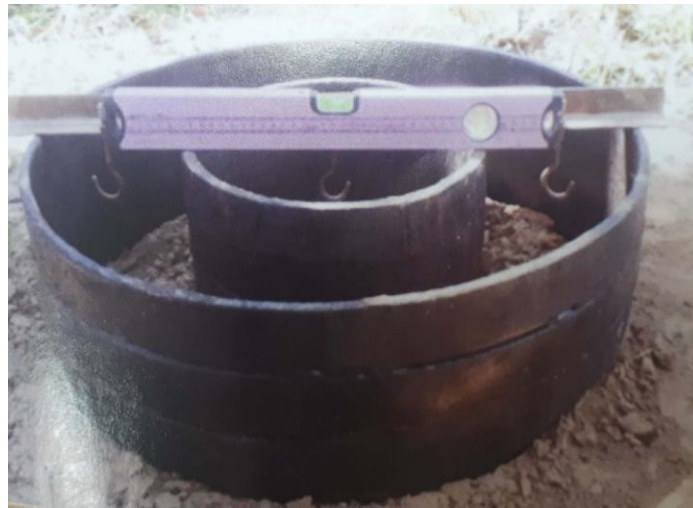
Figure 3.11: Picture courtesy by Malik et al. , 2019 (PCRWR) An angle with steel bar provided with steel hooks and a spirit level for leveling the infiltration rings and maintaining water depth
