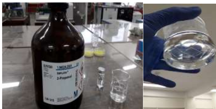
Figure 3.4: Cleaning of Substrate with 2-Isopropanol and Acetone
