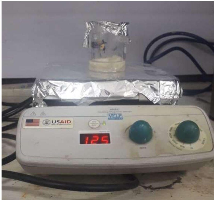
Figure 3.2: Stirring of the solution on a hot plate at control temperature and RPM
