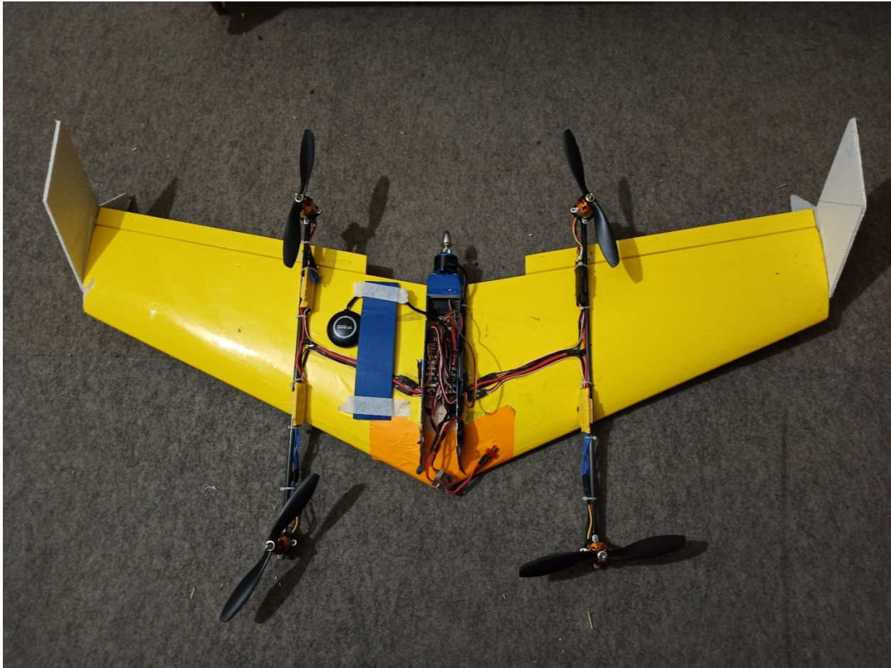
Figure 39. VTOL after attaching all components except back propeller
