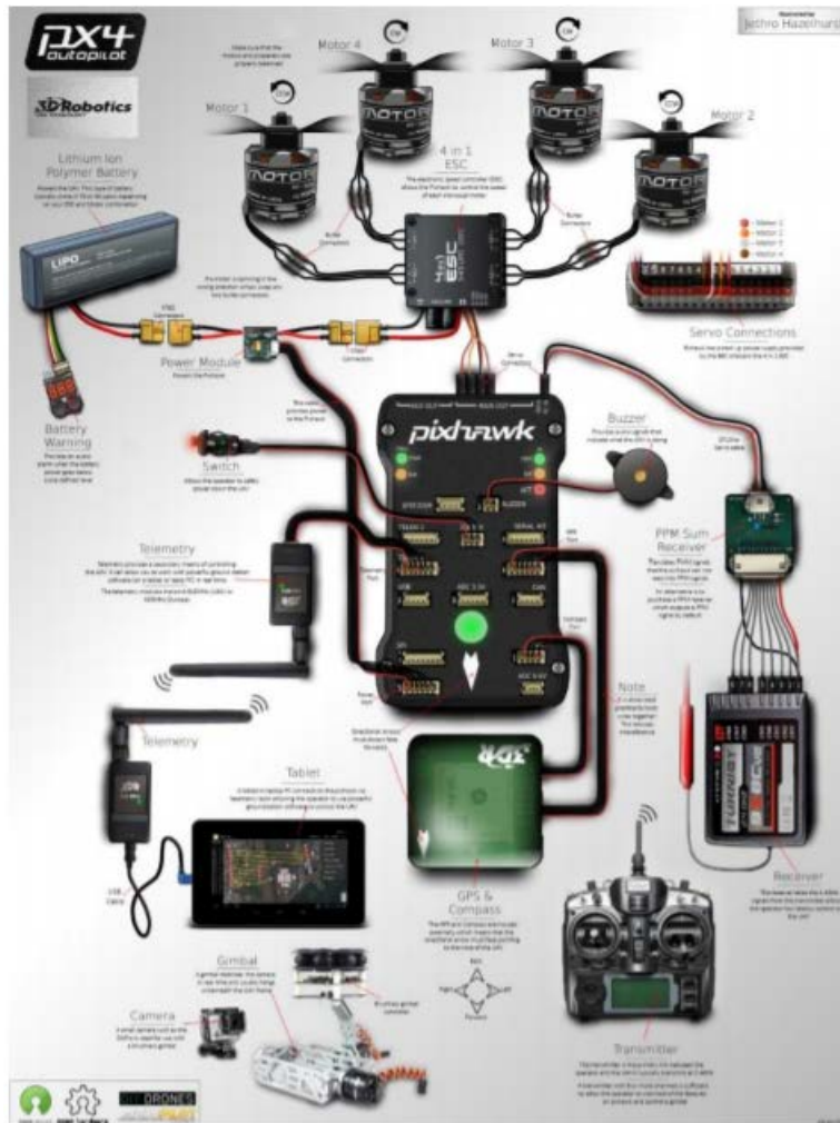
Figure 4. Pixhawk Components and structure
